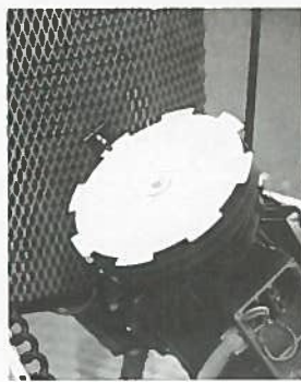
A rotating disc, with optical pick-up, produces the music.
