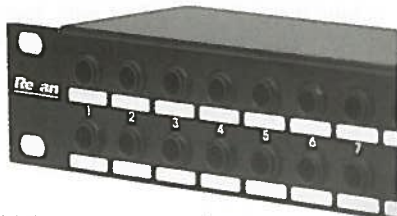
Solid nickel silver, self cleaning high tension contacts, NO SOLDER SET-UP - de normalise by rotating channel card. Re'an jacks. Formulated nylon and fibreglass composite, rated for over 10,000 Insertions
