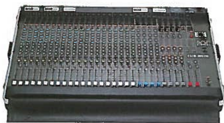
RCS2842 28 channel stereo mixing console *SKB custom-fit road case *46 inputs * 4 sub groups *8 aux sends *3 & 4 band EQ * master inserts *mute & PFL for 8 stereo aux returns.
