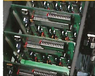
Full cyan/magenta/yellow colour mixing. Below: modular electronic system with built-in switch-mode power supply PCB
