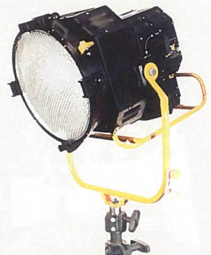
The Remington 1200W discharge daylight open-ended Par light using a single-ended MSR lamp. The range now covers 200W to 6kW and all have a removable lens system.
