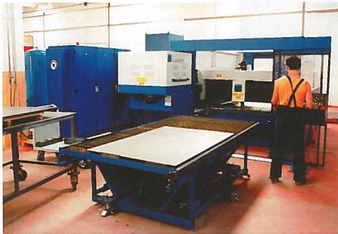
DeSisti employ the latest programmable laser cutting technology.
